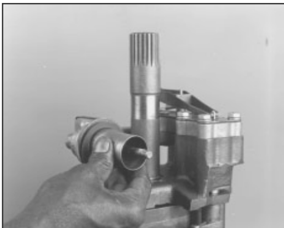
9. Remove the strainer inner shroud (fig 48).
