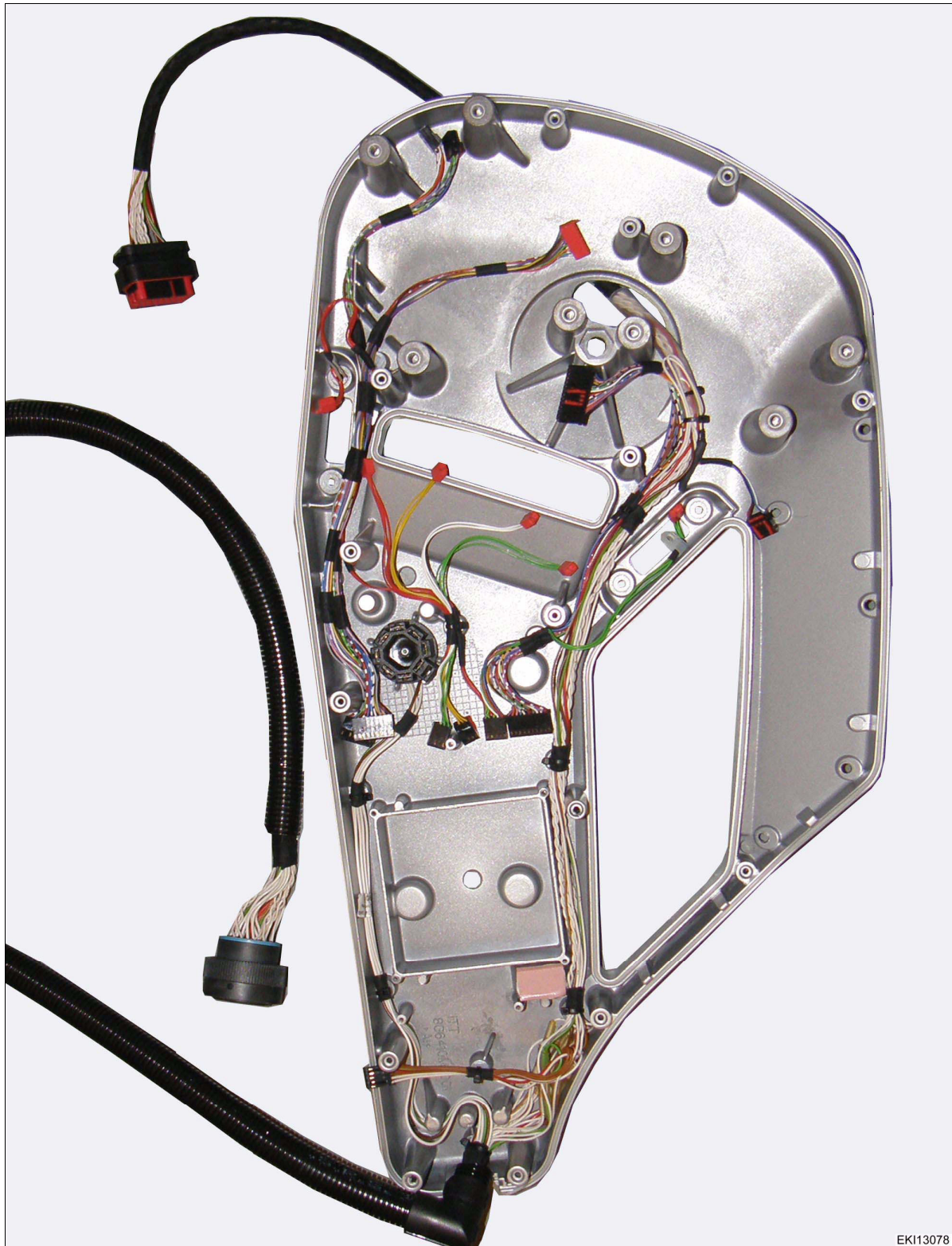
Fig. 80. Carefully route the wiring harnesses. Make sure that no chafing points develop.
