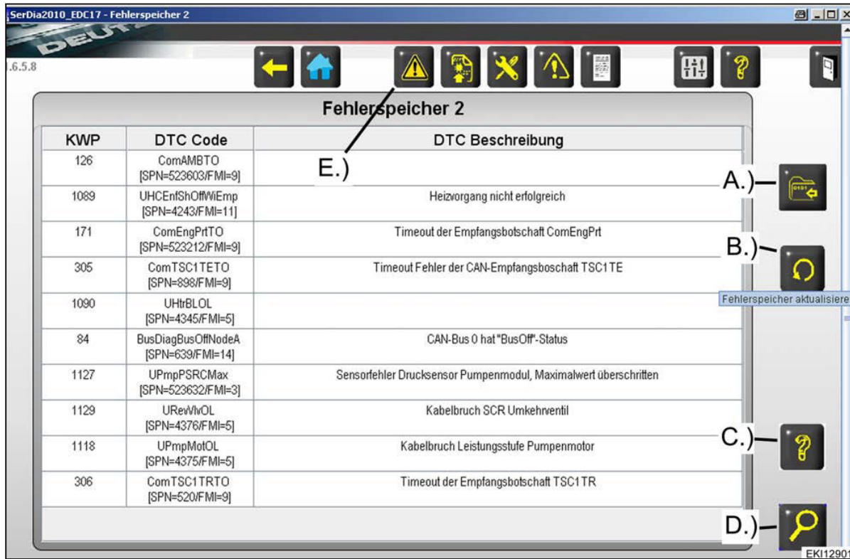
Fig. 19 This opens fault memory 2 (not deletable)
