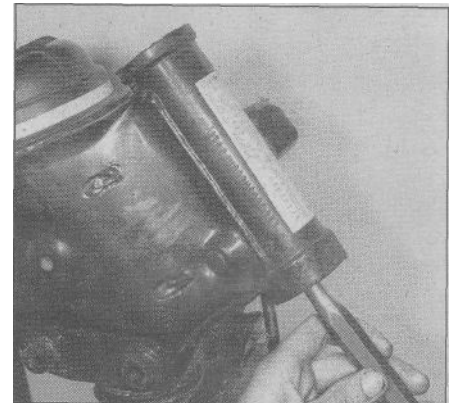
6.10a Insert a long punch or rod from below to tap out the upper bearing bottom race ...
