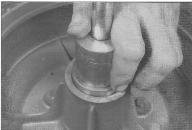
13.16e Make sure the spacer and collar are in place, then drive in the bearing on the opposite side
