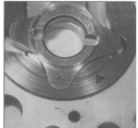
15.7f Note the marks on the rotors; they must face in the same direction when the pump is assembled .
