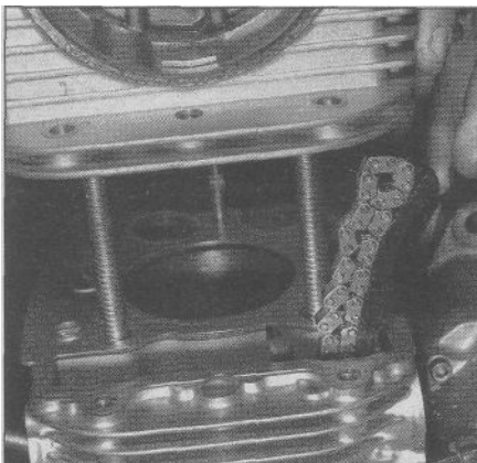
8.46a As you lower the head onto the studs, move the cam chain and damper aside so they don't obstruct installation of the head
