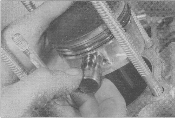
12.4a Push the piston pin partway out, then grasp it and pull it the rest of the way
