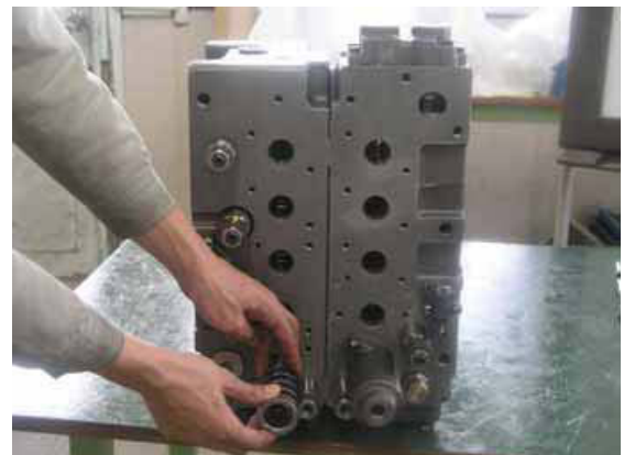
Fig. 33-163 Disassembling arm 2 spool (308) assy
