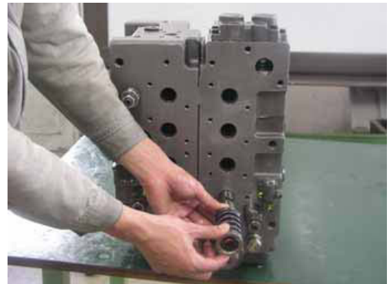
Fig. 33-161 Disassembling arm 1 spool (302) assy
