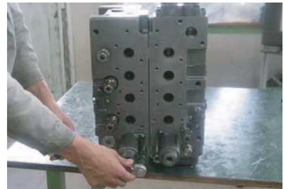
Fig. 33-162 Removing arm 2 spring cover (201)
