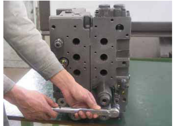
Fig. 33-160 Removing arm 1 spring cover (201)
