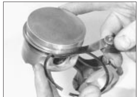
11.17 Measuring the piston ring-to-groove clearance
