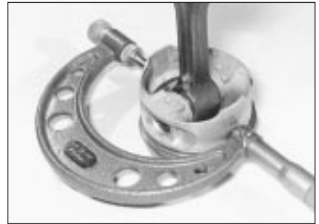
11.16 Measuring the piston diameter
