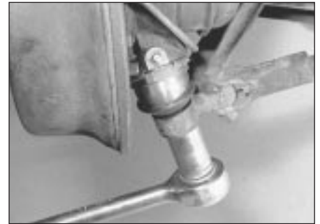
3.6 Remove the lower swivel hub balljoint retaining nut
