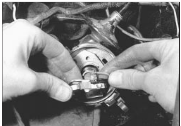
6.10b The LT terminal can then be detached from the tensioning arm
