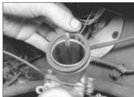
2.2b Recover the sealing ring
