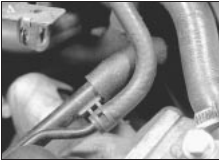
8.19a Disconnect the two vacuum/breather hoses from the left-hand end of the cylinder head . . .
