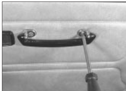
6.1 Remove the interior pull handle retaining screws and handle
