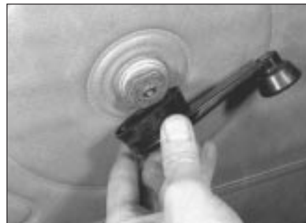
6.2b . . . and the window regulator handle
