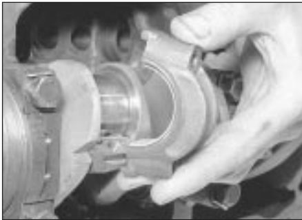
11.3 Removing a connecting rod big-end cap
