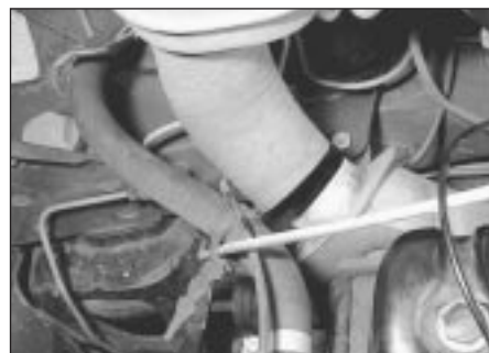
2.3a If the air cleaner is retained by two wing bolts detach the hot air duct . . .
