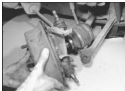
3.9 Withdraw the swivel hub from the end of the driveshaft
