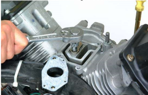
Figure 9-39. Removing Breather Reed.
