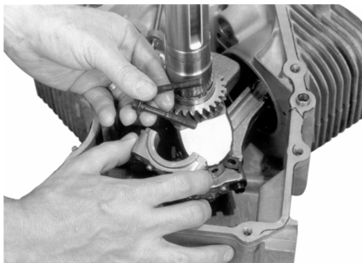
Figure 11-10. End Cap and Rod Bolt Detail.
