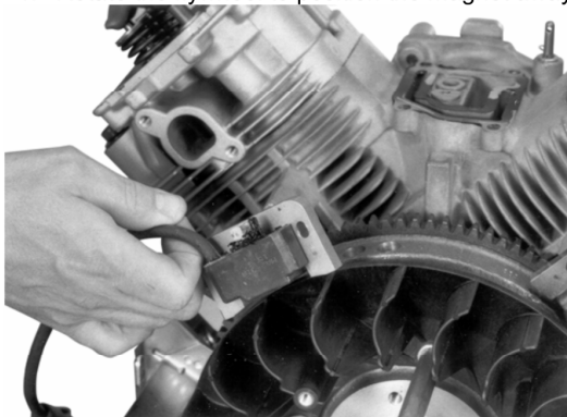
Figure 11-49. Installing Ignition Module.
