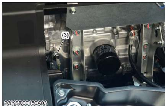
(3) Oil pressure switch
