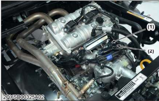
(1) TMAP sensor (2) 4P connector
