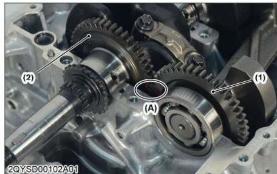
(1) Balancer shaft (2) Crankshaft (A) Timing marks
