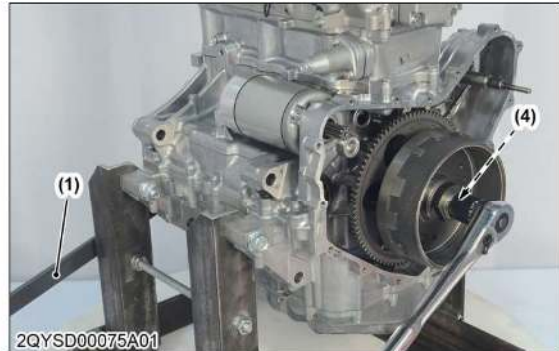
(1) Clutch holder (4) Flange nut
