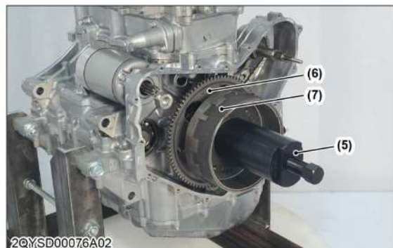
(5) Flywheel puller (7) Flywheel (6) Starting gear
