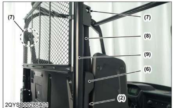
(1) Rear ROPS plate (6) Center upper cover (2) Flange bolt (7) Lock nut (3) Rear ROPS bolt (8) Seat belt (4) Flange bolt (9) ROPS (5) Lock nut
