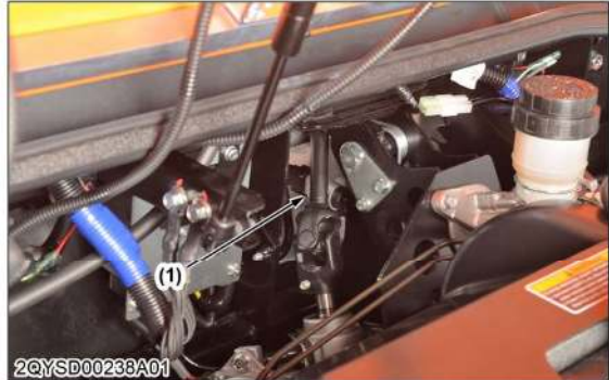
(1) Brake lamp switch
