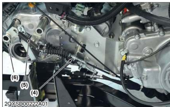
(1) Differential lock pedal (2) Adjusting nut (3) Differential lock cable (4) Adjusting nut (5) Differential lock spring (6) Differential lock lever
