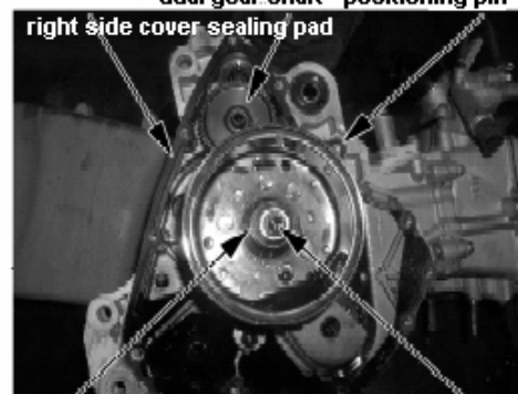
nut and washer spring of oil duct connector
