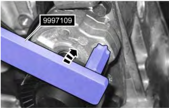
Fig. 372: Identifying Belt And Special Tool 999 7109 Courtesy of VOLVO CARS CORPORATION
