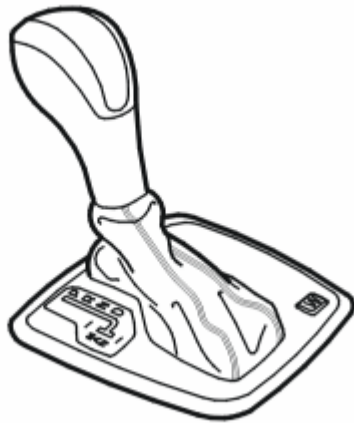
Fig. 316: Identifying Automatic Transmission Gear Shifter With Manual Gear Changer Courtesy of VOLVO CARS CORPORATION
