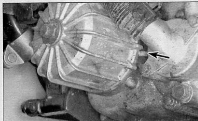
11.7 Position the filter tabs on either side of the water pump cover boss (arrow)
