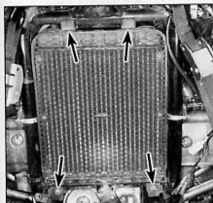
7.6a The radiator is secured by nuts and studs at the bottom and tabs at the top (arrows); the stone shield is secured to the radiator by six bolts
