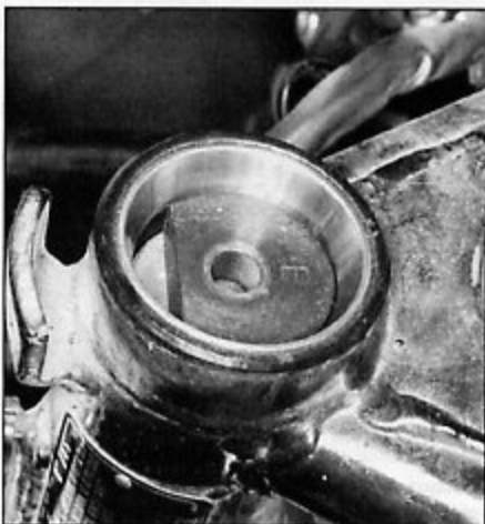
7.11a This Honda tool fits into the upper bearing race; tapping the tool upward from below will push the race out
