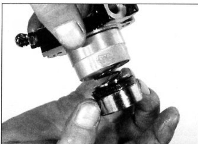
13.26 Take the piston and spring out of the cylinder and remove the seal from the piston; the wide side of the seal faces into the bore
