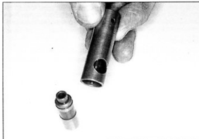
9.37 This tool opens the check valve in the lash adjuster so it can be filled with kerosene
