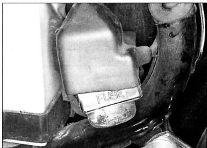
5.1c The main fuse is located next to the battery
