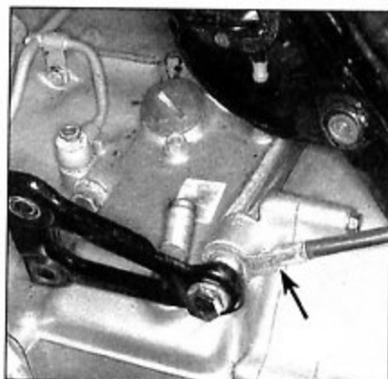
5.20c . . . the through-bolt, which connects the left and right engine mounts, secures a ground cable (arrow) on the left side
