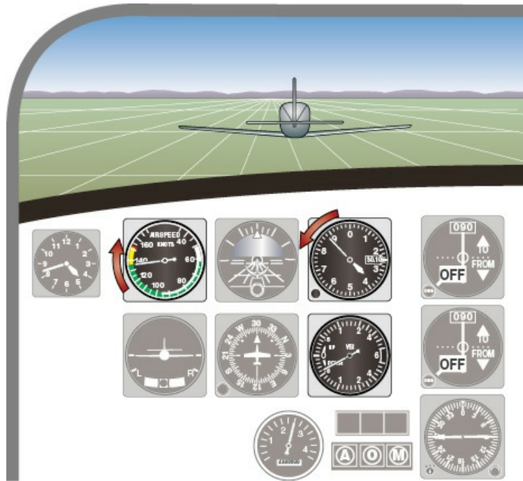
Figure 4-2 The vertical performance instruments showing a gradual loss of altitude and airspeed increase.
