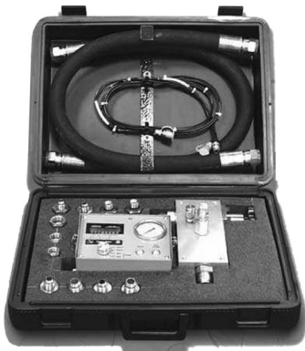
Hydraulics test set
