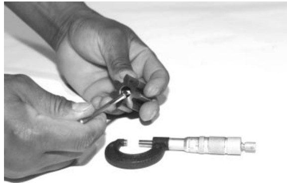
Measure Idler Gear ID for Wear
