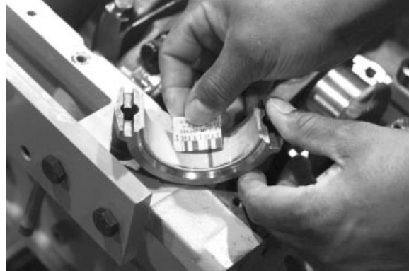
Measure Rod Oil Clearance
