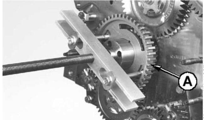
Remove Timing Wheel
