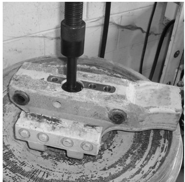
Front Idler Shaft Removal
