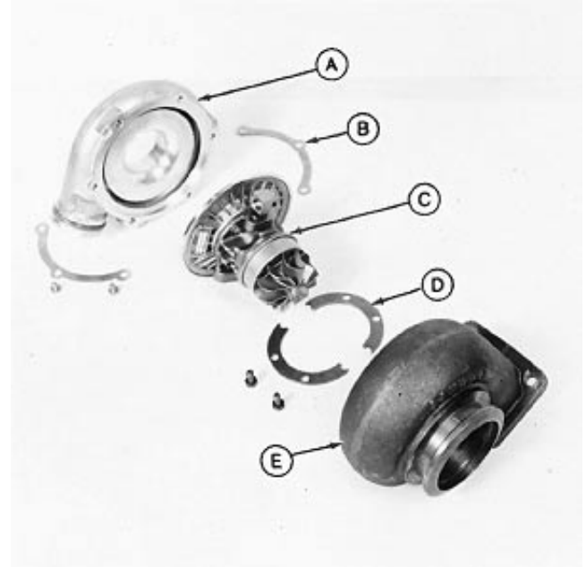
A—Compressor Housing B—Clamp Plates C—Center Housing Assembly D—Clamp Plates E—Turbine Housing
