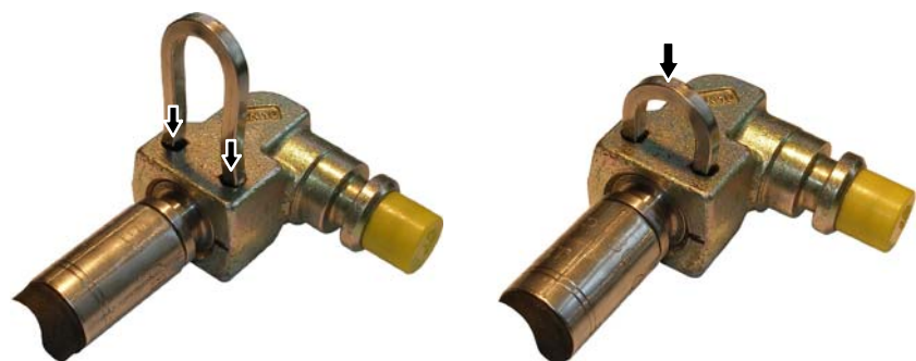
Fig. 9: Press the staple together to align the ends with the holes and pound it in
