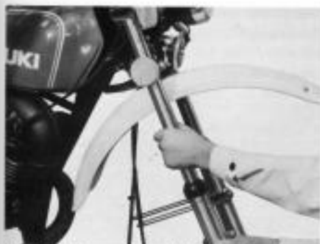
Fig. 10-7. Remove front fork by drawing it out.
