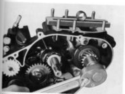
Fig. 7-46. Using special tool (part No. 09910-20115), remove primary drive gear nut and take off drive gear.
