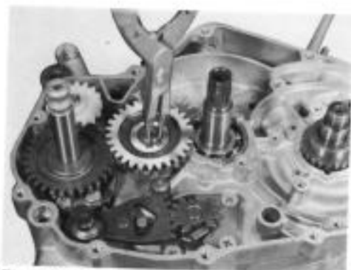
Fig. 7-48. Using special tool (part No. 09920-70111), remove circlip, and draw out kick starter idle gear.
