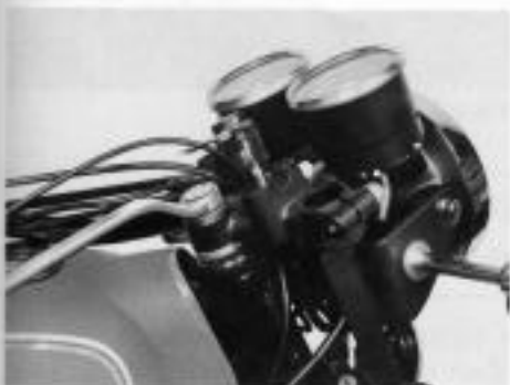
Fig. 10-8. Remove steering stem upper bracket by loosening the stem bolt.
