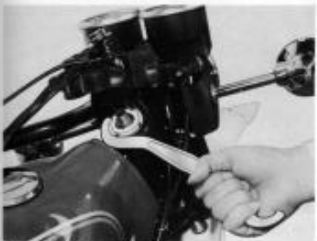
Fig. 10-9. Remove steering stem nut with special tool (part No. 09940-10122), and slide off the stem. Be careful not to let the steel balls fall off.
