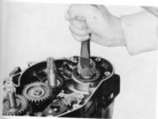
Fig. 7-45. Flatten primary drive gear washer.
