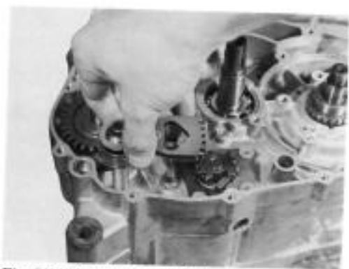
Fig. 7-49. Pull out gearshift shaft.
