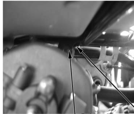
Bolt 2, Upper Engine Hanger Nut 2, Upper Engine Hanger
