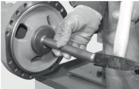
FIGURE 2: Insert the thrust block (6) and the shims (Sb)(7) into the arm.
