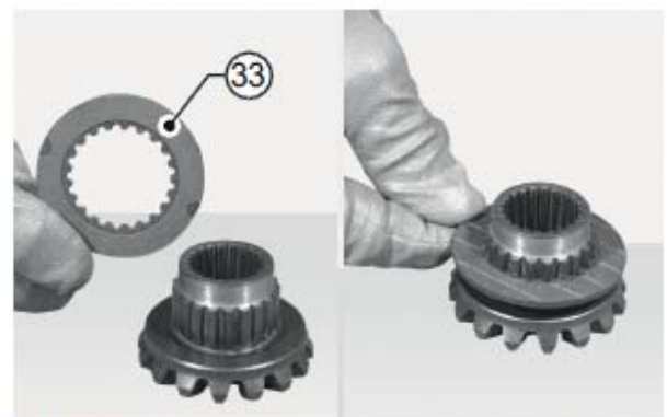
FIGURE 23: As to ring (33), the side without notches must face outwards.
