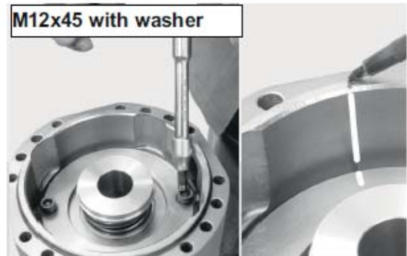
FIGURE 9: In order to keep the disc springs of the negative brake preloaded, tighten the screws with washers to the end stop.
