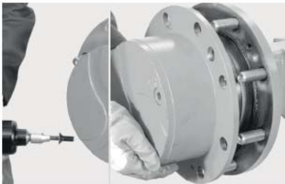
FIGURE 5: Remove the screws of the planetary gearbox cover on the brake side. Remove the planetary gearbox cover.
