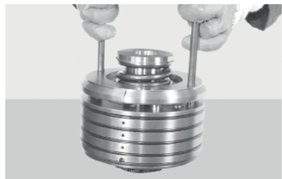
FIGURE 65: Insert two screws of M12 to fix the break arm.
