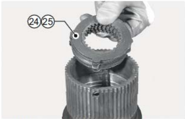
FIGURE 20: Insert and replace, if necessary, the discs of the differential lock (24, 25). In case of new discs pack (as spare part), dip the complete disc pack in oil (with LS additive) at least 8 hours (plus 2 dripping hours) before assembly, for details about oil see MAINTENANCE INTERVALS p. 20
