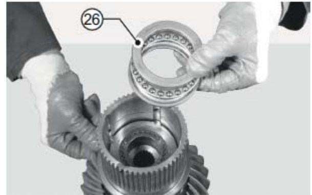
FIGURE 21: Install the thrust block with maximum internal diameter. Position the bearing (26) in the differential unit. Install the thrust block with minimum internal diameter.
