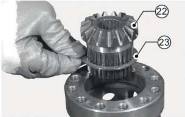
FIGURE 12: Remove the planetary gear (22) with washer (23).
