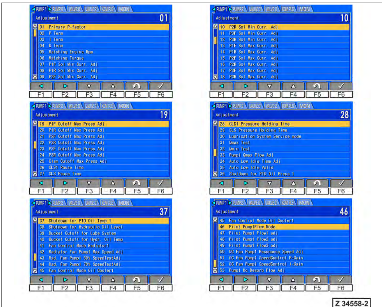
Fig. 16-104 Adjustments for PUMP1 controller
