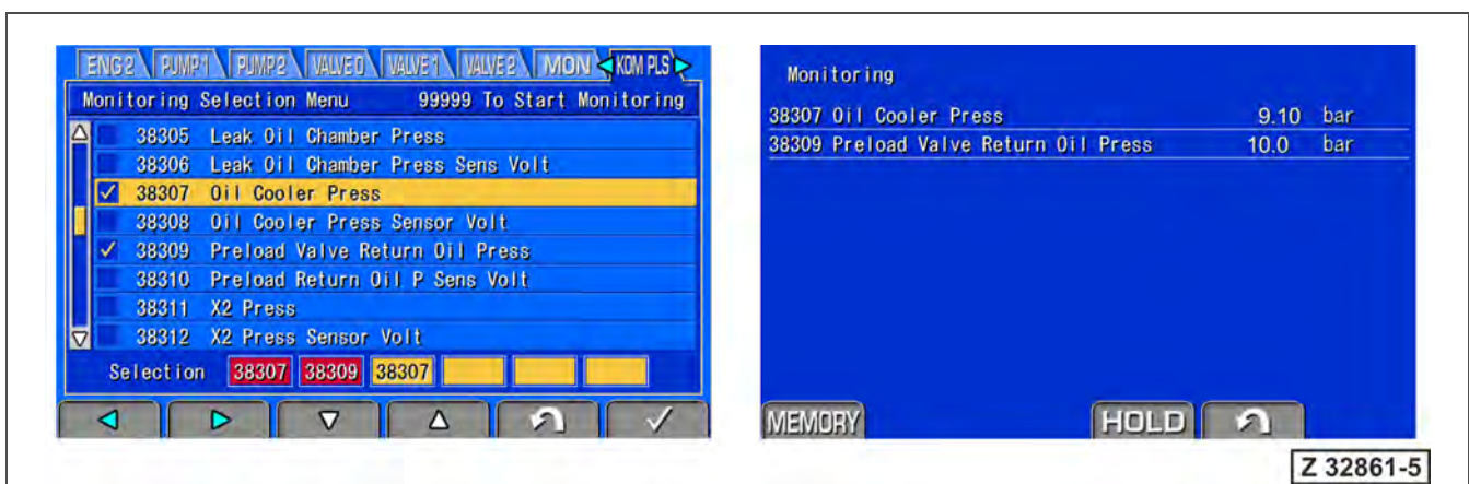
Fig. 6-18 Monitoring screens for 40B165 and 40B166
