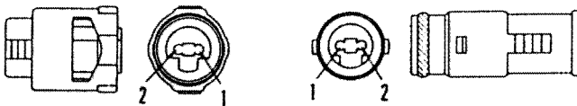
CN-C20 (Front engine TVC solenoid) ECONOSEAL connector 2 pins CN-C23 (Rear engine TVC solenoid) ECONOSEAL connector 2 pins
