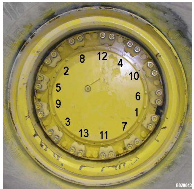
FIGURE 2-8. REAR TIGHTENING SEQUENCE
