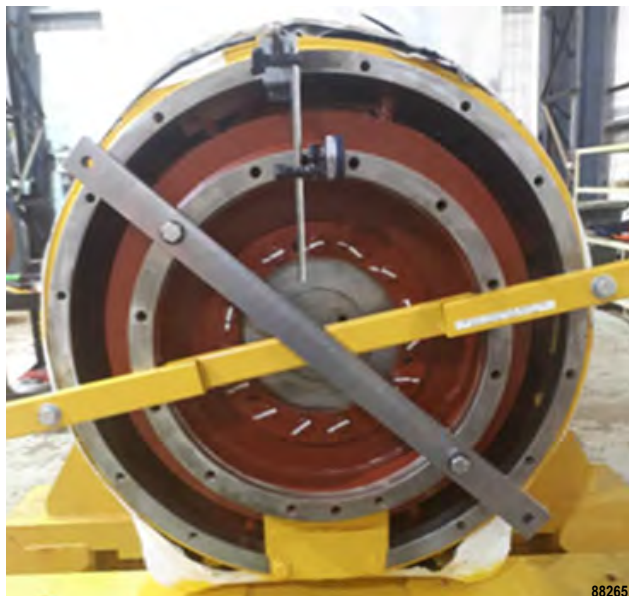
FIGURE 50-35. ALTERNATOR HOUSING TO ROTOR MEASUREMENT
