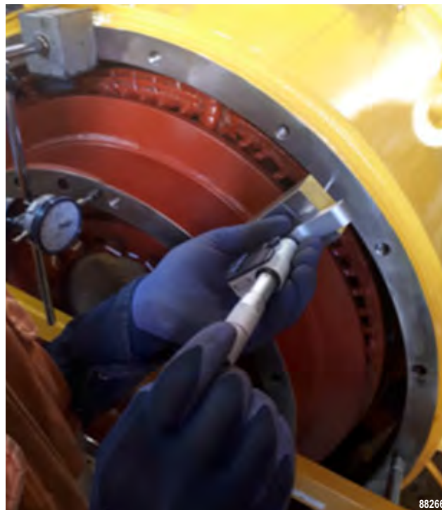
FIGURE 50-36. ALTERNATOR HOUSING TO ROTOR MEASUREMENT
