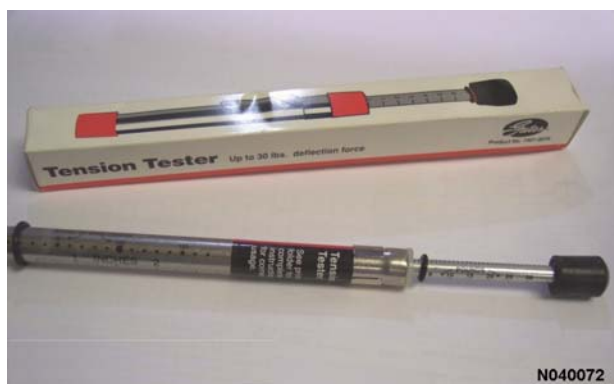
FIGURE 4-13. BELT TENSION TOOL - XA3379
