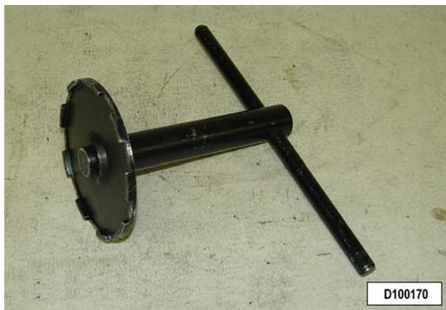
FIGURE 10-24. XA3320 FIELD COIL REMOVAL/INSTALLATION TOOL
