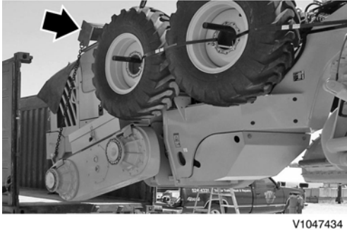
Figure 5 Using a spreader bar to lift the rear of the machine
