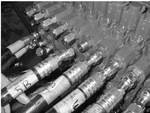
Figure 6 10 bank hoses, remove & cap
