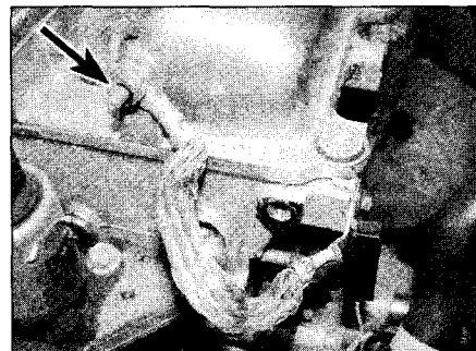
5.9b . . . then undo the earth strap retaining nut (arrowed)
