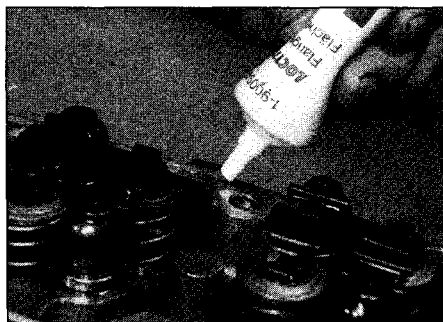
12.25 Apply sealant to the cylinder head upper mating surface then refit the camshaft housing
