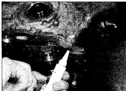
12.10a Apply a smear of sealant to the areas of the cylinder block/timing chain cover joints . . .
