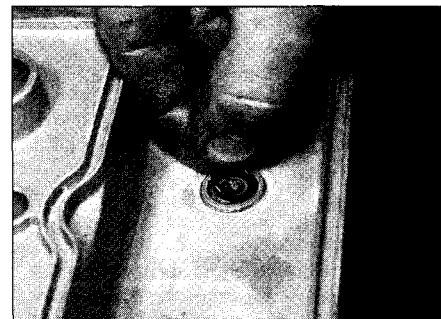
4.6b ... and fit the sealing rings to the recess around each retaining bolt hole
