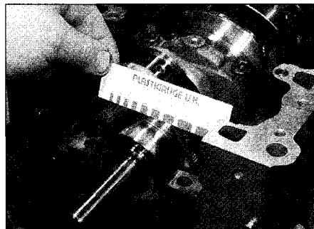
18.9 Measure the width of the deformed Plastigauge using the scale on the card
