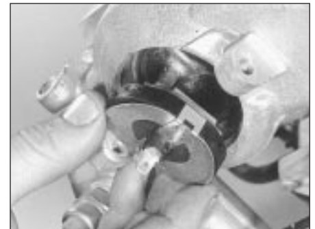
15.7b . . . and remove PTC heater from inlet manifold - manifold removed for clarity
