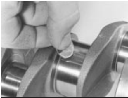
14.6 Using a penny to check crankshaft journal condition
