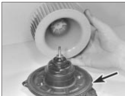
10.20e . . . and lift off fan (seal arrowed)
