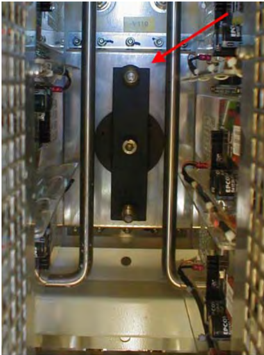
FIGURE 10-43. FREE-WHEELING DIODE FOR LOW-INDUCTANCE BUS BARS, FRONT VIEW
