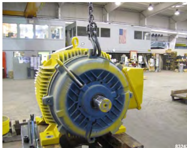
FIGURE 50-21. LIFTING THE BEARING HOUSING
