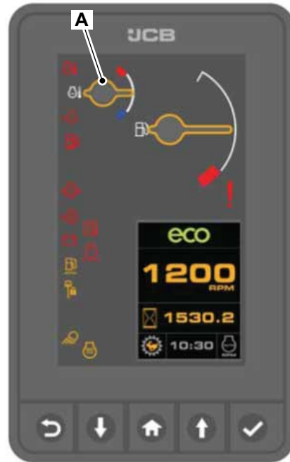
A Coolant temperature gauge
