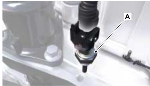
A Coolant temperature sensor
