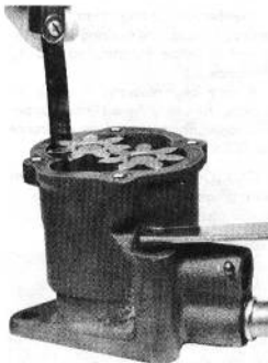
FIGURE 34 — Measuring Oil Pump Gear to Body Clearance
