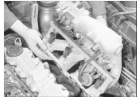
38.14B ...and withdraw the inlet manifold - SOHC models
