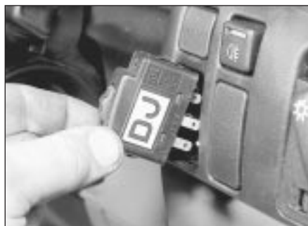
27.4 The headlamp aim adjustment switch - 1992-on models
