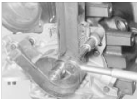
11.17A Loosening the main rear timing belt cover lower securing bolt - 2.0 litre engine
