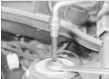
4.7 Unscrewing the suspension strut top mounting nut
