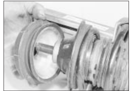
4.13A Lift off the strut upper mounting rubber . . .
