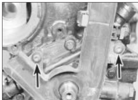
11.17B Main rear timing belt cover lower securing bolts (arrowed) - 1.6 SV engine
