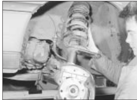
4.8 Withdrawing a suspension strut
