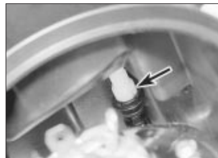
26.2B Headlamp aim adjuster balljoint (arrowed)
