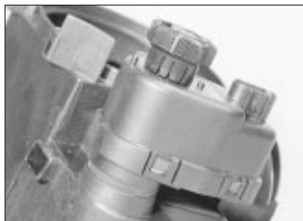
26.2A Headlamp aim adjustment motor (headlamp removed)
