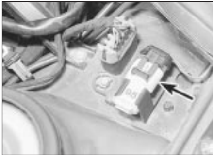
22.3 Octane coding plug (arrowed) - 2.0 litre model
