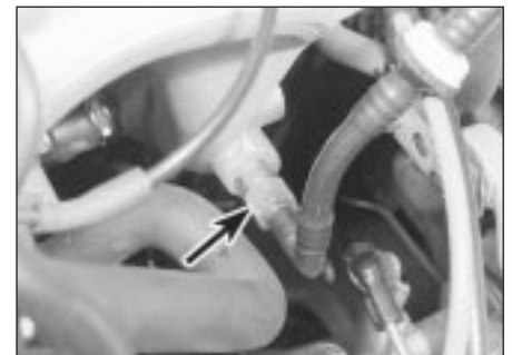
40.13 Brake servo vacuum hose connection at inlet manifold (arrowed) - DOHC models
