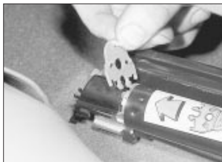
43.4 Inserting the safety fork into the aperture in the seat belt tensioner spring cylinder
