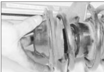
4.14 Lift off the upper spring seat and damper ring
