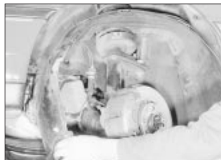
31.1 Removing a wheel arch liner
