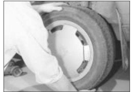
5.4 Check for wear in the hub bearings by grasping the wheel and trying to rock it
