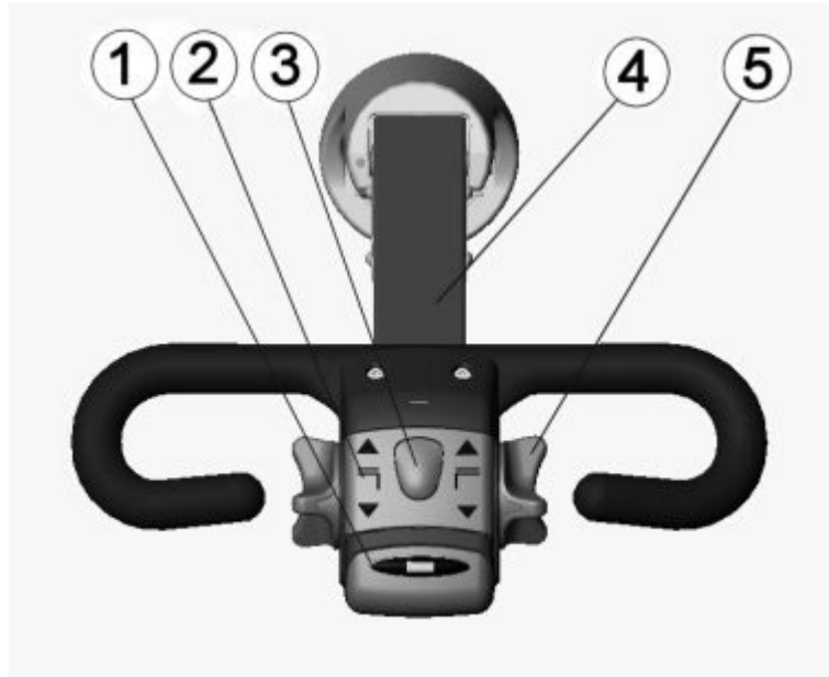
Figure 2.2. Tiller arm controls
