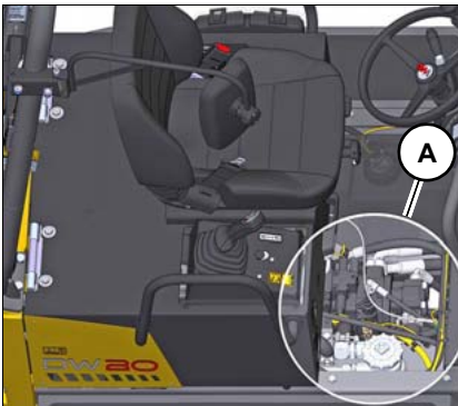
Fig. 34 Hydraulic pump access
