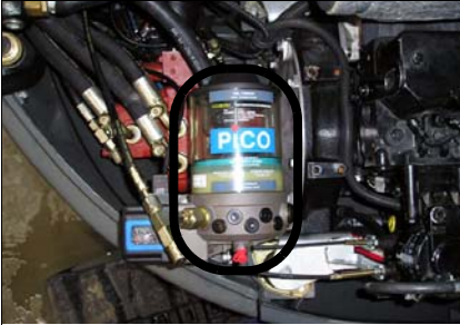
Fig. 11: Central lubrication system pump
