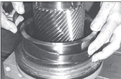
Fig. 25: Removing the seals and bearings
