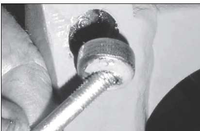
Fig. 27: Removing the grease nipple, etc.
