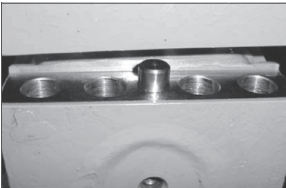
Fig. 67: Installing the parallel pin in the base block
