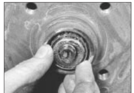
6.5c ... and outer bearing
