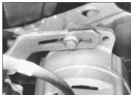
13.4a Alternator drivebelt tensioner link - 1.3 litre
