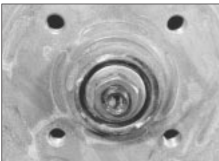
6.5a Undo the hub nut ...
