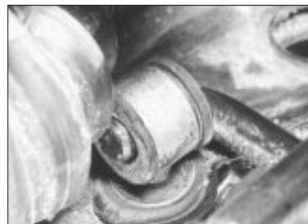
4.5 Anti-roll bar location in eye bolt
