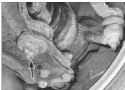
4.2 Anti-roll bar eye bolt nut (arrowed)
