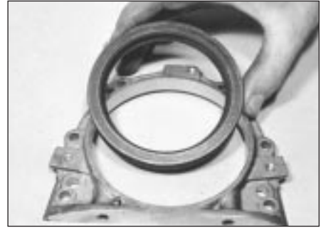
14.14 Remove crankshaft rear oil seal from housing
