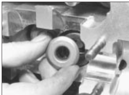
5.10 Removing valve spring upper seat
