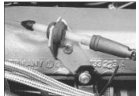
8.10 Accelerator cable adjuster and support bracket
