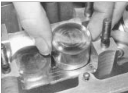
5.4 Removing an hydraulic bucket tappet
