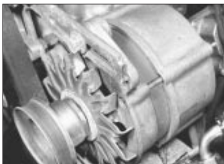
13.4b Alternator drivebelt tensioner link - 1.8 litre
