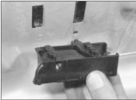
15.3 Removing interior door handle and finger plate
