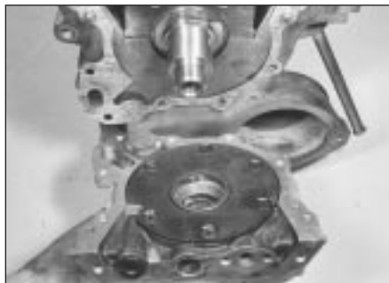
16.4a Removing oil pump . . .
