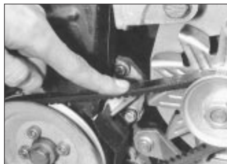
13.2 Checking alternator drivebelt tension
