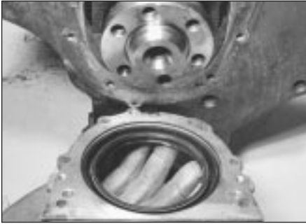
14.13a Withdrawing crankshaft rear oil seal housing . . .
