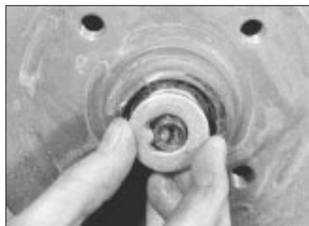
6.5b ... remove the thrustwasher ...
