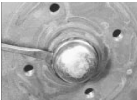
6.4a Remove the hub cap ...
