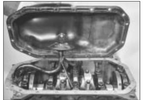
15.2 Removing the sump
