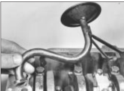
16.3 Removing oil pump pick-up tube and strainer
