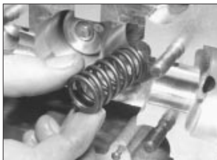
5.11b Removing an inner valve spring
