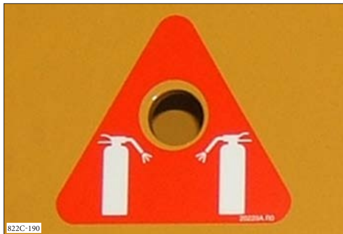
Typical Fire Extinguisher Access Port
