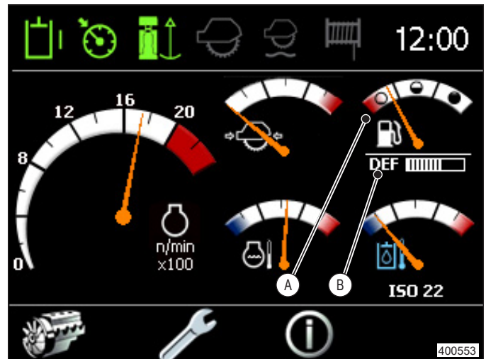
A Fuel Level Gauge B DEF Level Gauge (Tier 4f Machines Only)
