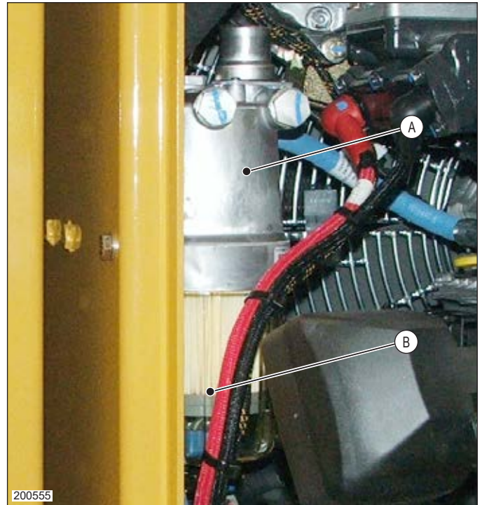
A Fuel Filter/Water Separator B Fuel Heater (Bottom of Clear Bowl)
