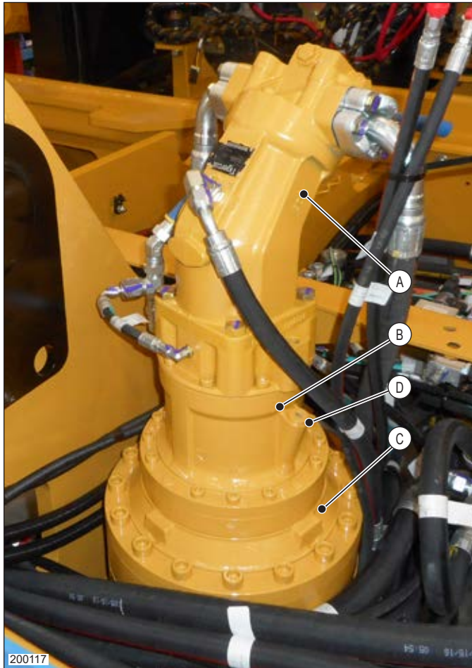
200117 A Swing Motor B Swing Brake (Optional) C Swing Drive Gearbox D Fill Plug–Swing Brake Housing (Optional)
