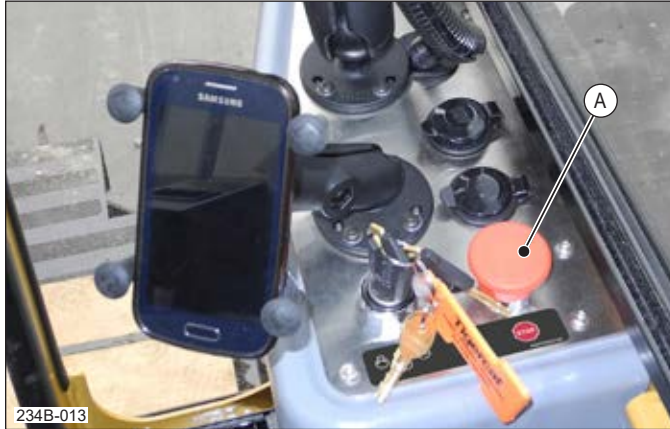
A Emergency Stop Switch
