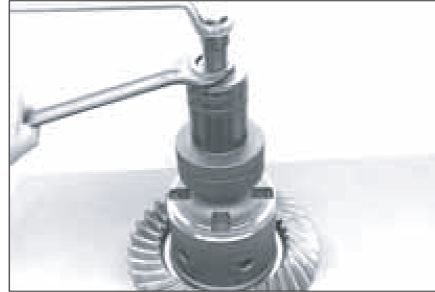
Pull bearing inner ring from the differential housing.
