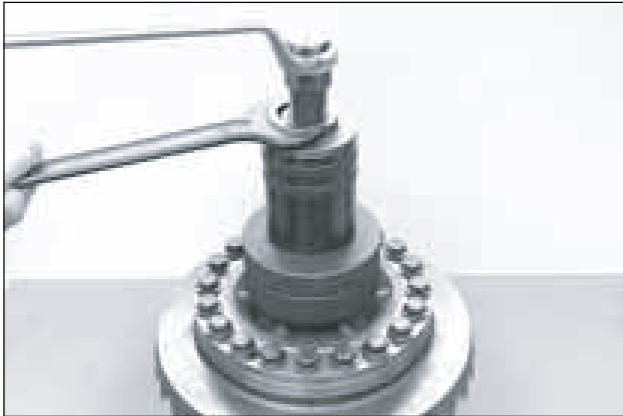
Pull bearing inner ring from the housing cover.
