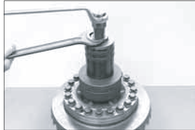
Pull bearing inner ring from the housing cover.
