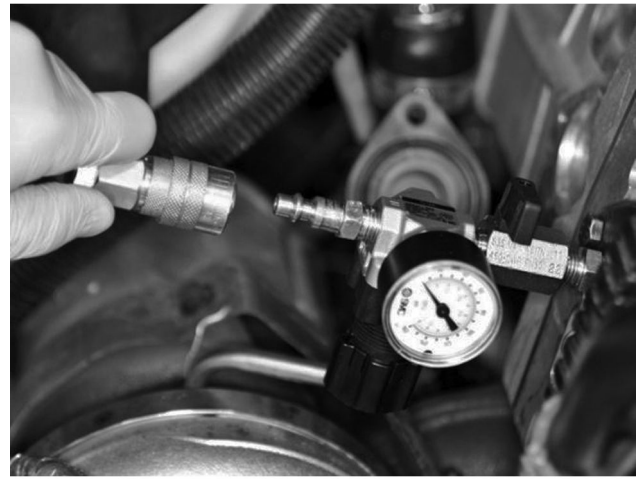
Figure 343 Shop air hose removal
