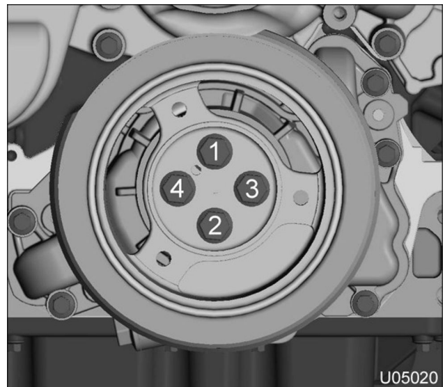
Figure 404 Torque Sequence for Vibration Damper Bolts
