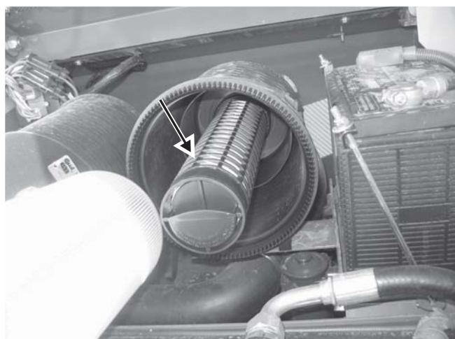
Fig. 10-14 View of the safety filter element inside of the primary filter element.
