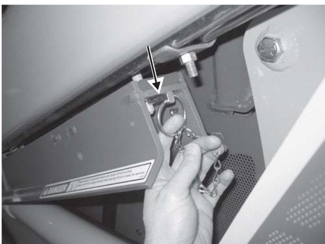
Fig. 2-3 Pull ring out of welded post.
