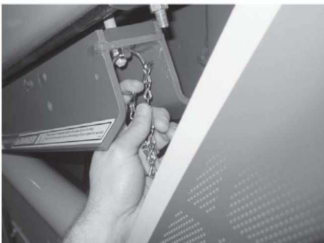
Fig. 2-2 Flip lock pin down and grab with finger.
