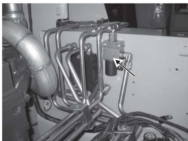
Fig. 8-24 Location of the lift solenoid ( 2086 Models).
