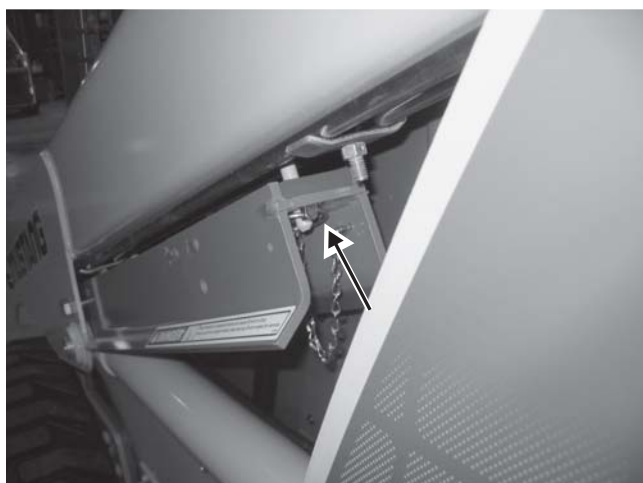
Fig. 2-1 The lock pin secures the liftarm support device underneath the left liftarm.
