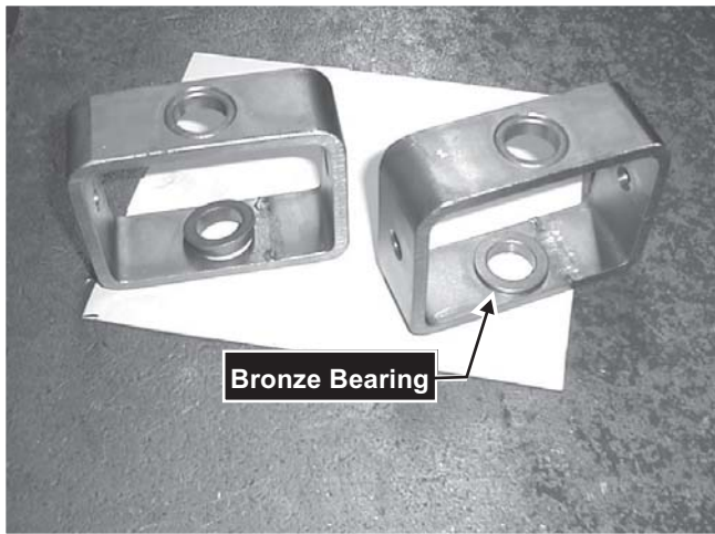
Fig. 6-16 The left and right control handle pivots are identical.
