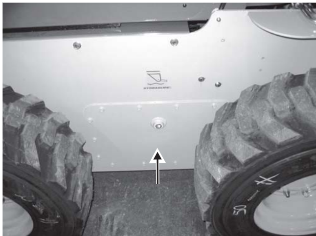
Fig. 7-15 Remove chaincase cover to access drive chains on both sides of the loader.
