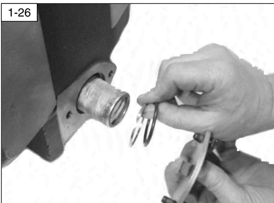
1-26 Remove 2 screws and withdraw the strainer cover, O ring, spacer and strainer.
