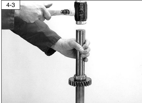
Using an appropriately sized tube replace the front and rear bearings.
