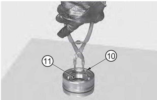
FIGURE 7: Fit the snap ring (10) on the bearing (11).
