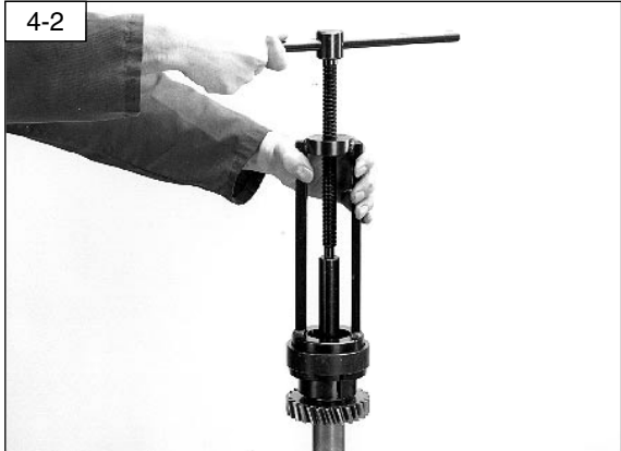
Using the appropriate bearing puller remove the front and rear bearings.
