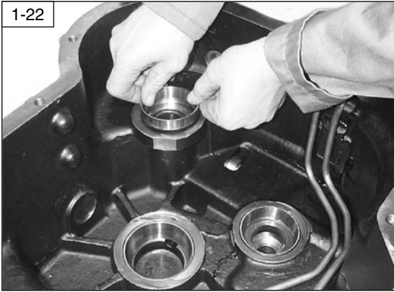
1-22 Remove the bearing shells from the front case.
