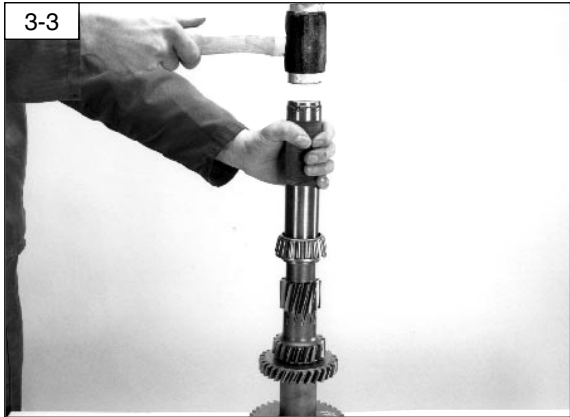
Using an appropriately sized tube replace the countershaft front and rear bearings.
