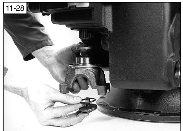
11-28 4WD VERSION : Replace the spacer, 4WD yoke, "O"ring, washer and bolt. Then tighten to a torque of 50 to 65 lbs / ft.
