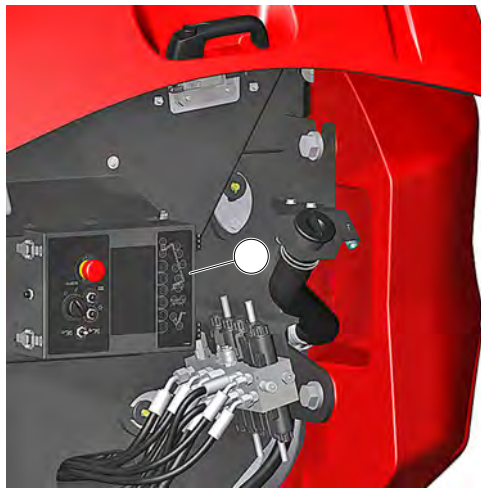
Figure 116: Location of ground control panel Fuses/Relays box
