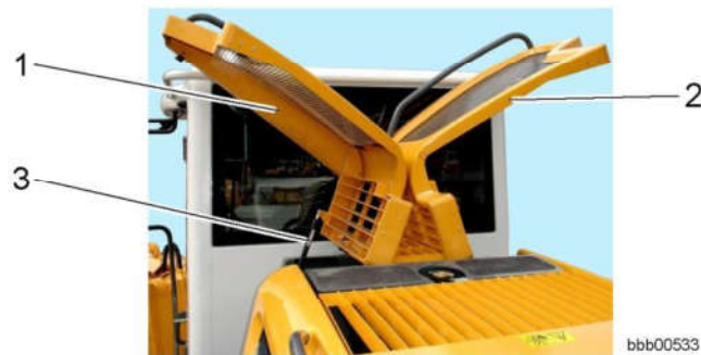
Cooling system hood
