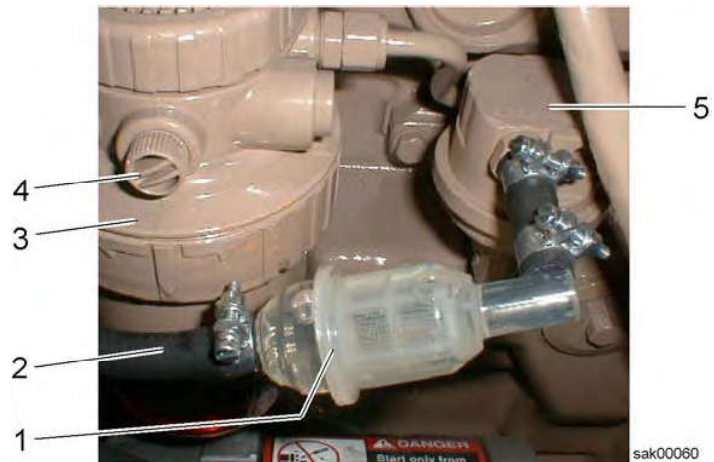
Fuel pre-filter installation
